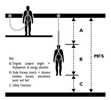
As all testing of energy absorbing Lanyards is based on a 100kg mass, we offer the following guidance for users over 100kg.
